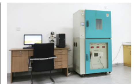
模拟EV车高频电晕老化试验仪器 Simulation EV vehicle high frequency corona aging test equipment
