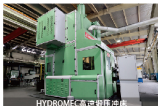
HIGH-SPEED FORGING PRESS EQUIPMENT
